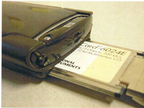
b. Insertion of DAQ card into PDA expansion pack
