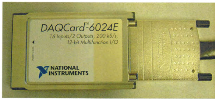
a. DAQ card – data cable connection
